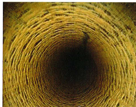
Stainless Steel Tube with Scale Deposits
