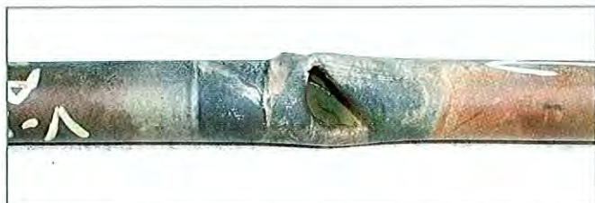
Figure 5: Admiralty brass tube, failed by impact damage due to unknown object propelled into condenser at startup, after turbine outage.
