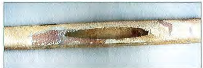
Figure 6: Admiralty brass tube, failed by drain line erosion due to failed valve.
