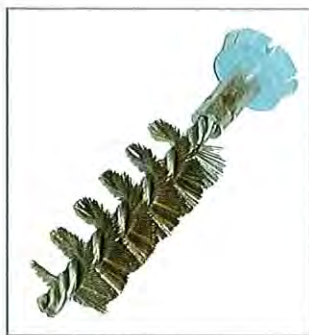
Figure 3: Stainless Steel Tube Cleaning Brush, for general purpose tube cleaning, including when scrapers will not fit properly due to inlet-end inserts or epoxy coating (Conco Systems, Inc.).
