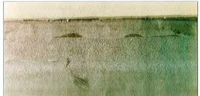
Figure 19: 304 stainless steel tube with defects at incompletely formed weld seam. Magnification 4x.
