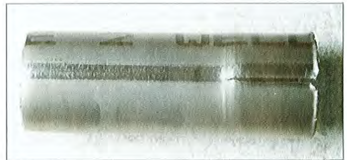
Figure 21: Titanium tube that failed at weld seam upon rolling into tubesheet, due to manufacturing embrittlement, combined with freezing while filled with water during temporary storage.
