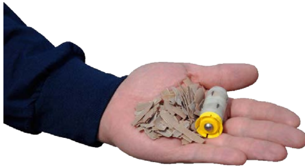
Figure 1: Scale as removed from condenser tubes
